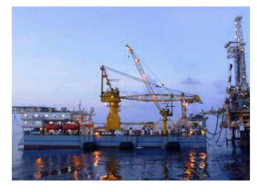
and is ideally suited to the fast paced Gulf of Thailand infield drilling programs. It can work in water depths of 6,000 feet (approx. 1,828 metres) and has a drilling depth of 20,000 feet
