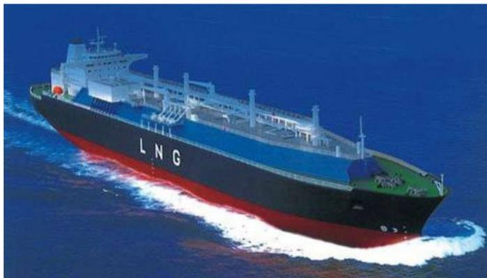
The vessel will be equipped with a dual fuel driven main engine and a controllable pitch propeller propulsion system. The efficient use of diesel oil and vapourized LNG during its transport greatly reduces energy loss and
