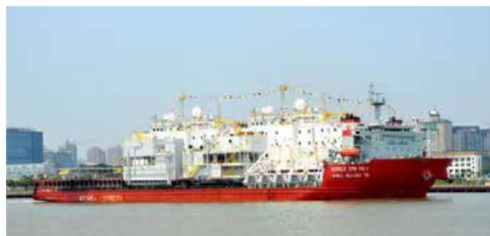
regulatory requirements. Among them, the four sets of living modules and generic modules represent the highest technology. Each living module measures 13.5 metres in length, 41.4 metres in breadth, 23.5 metres in height and 1,880 tons in weight, and fully adopt green design principles and outfitting materials, ergonomics and integration control technology, first-class air-conditioning systems and sanitary units and the most advanced internal and external communication systems.
